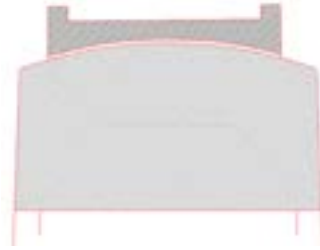
Front view of spherical bearing cut in half
